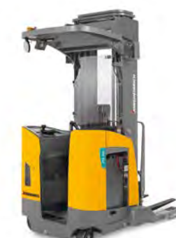
ETR 230-345d Pantograph reach truck max. lift height: 11,354 mm max. capacity: 2,000 kg
