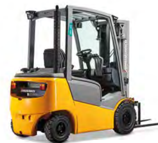
DFG/TFG 316-320 Diesel/LPG forklift truck hydrodynamic max. lift height: 7,500 mm max. capacity: 2,000 kg
