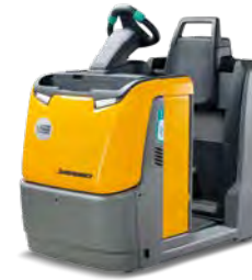
EZS 350 Tow tractor max. tractive power: 5,000 kg
