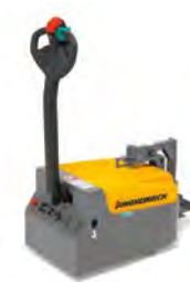
EZS 010 Tow tractor max. tractive power: 1,000 kg
