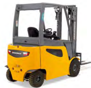
EFG 425-S30 Electric 4-wheel counterbalance truck max. lift height: 7,500 mm max. capacity: 3,000 kg
