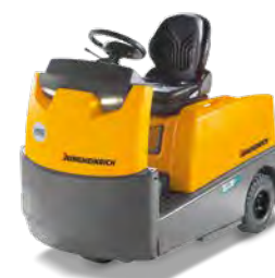
EZS 570-5100 Tow tractor max. tractive power: 10,000 kg
