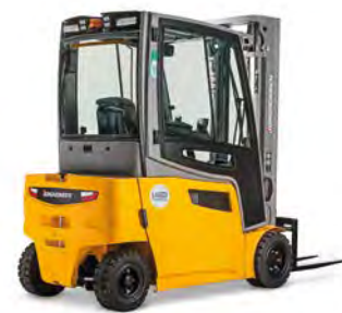
EFG 316-320 Electric 4-wheel counterbalance truck max. lift height: 7,000 mm max. capacity: 2,000 kg
