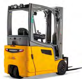
EFG 213-220 Electric 3-wheel counterbalance truck with front wheel drive max. lift height: 7,000 mm max. capacity: 2,000 kg
